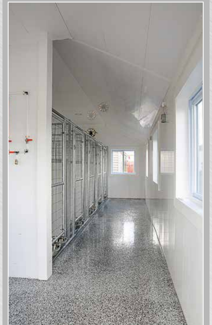
Interior View Of 10x28 5 Run kennel with 3' overhang with 10' Add on runs. Showing welded wire panels and exhaust fan.
